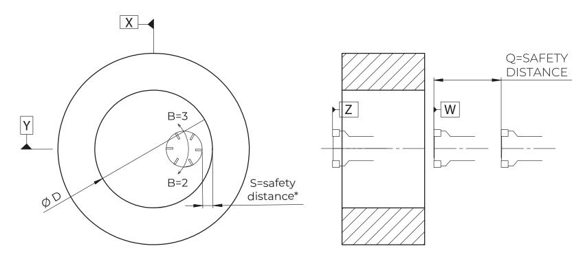
\* By setting S=0 the positioning before and after helical interpolation will be in the centre of the hole (only for internal contours U=1).
