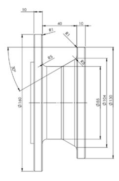
Roughing and finishing the closure with a front flange of a smaller diameter than the rear flange. Roughing the groove starts from the diameter of the lower flange, so it is a good idea to include turning cuts up to the diameter of the lower flange.
