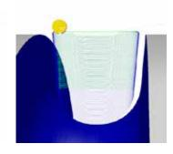
Recovery of the radius and the sides with transverse cuts
