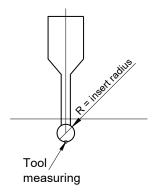
The R parameter is used to set the radius R of the tool, so there is no need to fill in the tool radius in the table, nor the T quadrant, as radius compensation is performed automatically within the macro.
