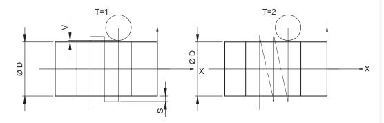
Parameter T is used to select the type of path to be followed in the lateral cuts: with T1 it will carry out continuous cuts with a return, while with T2 it will carry out cuts only in one direction, raising each time to the safety level and then carrying out the following cuts always in the same direction.
